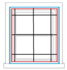
Using a steel tape measure inside the recess.
