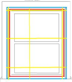
Measure using a steel tape measure outside the recess.
